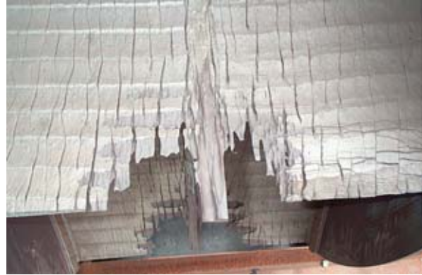
Figure 2. Fan Blades Protected by Chrome Carbide Weld Overlays after Twelve Months in Operation
