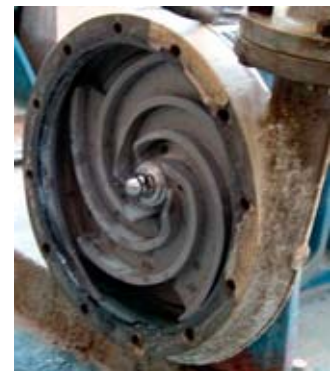
Figure 9. Slurry Pump Protected by Brazed Tungsten Carbide Cladding
