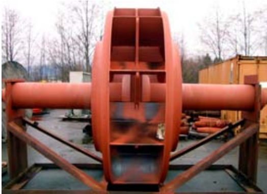
Figure 1. Port Alberni's Power Boiler ID Fan
