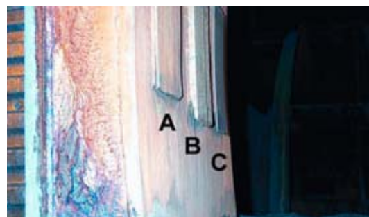
Figure 5. Comparison of Material Lengths after Six Months. A. Alloy Steel, B. Chrome Carbide Weld Overlay, C. Brazed Tungsten Carbide Cladding
