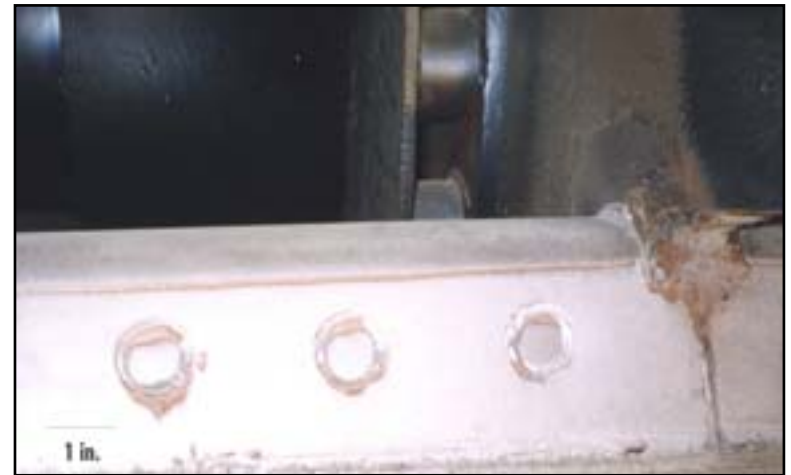
Brazed Tungsten Carbide Liner After 14 Months (no visible wear)
