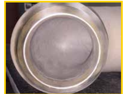
Return Bend Ready for Installation
